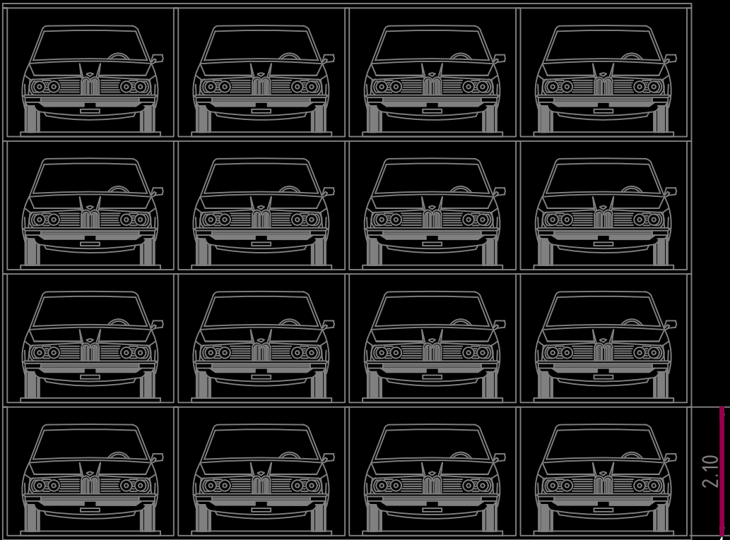
Mechanized Parking Level Height
